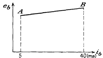
FIG. 14-17. A typical glow-tube volt-ampere characteristic.
